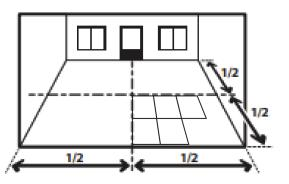
Installation shall commence from the intersection of the perpendicular axis. Tiles shall be laid true to the axis lines to ensure that they are laid square to each other. They shall be laid in a step or pyramid fashion to minimise tile creep.
